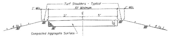
\* Note - Shoulders are not required when side slopes are less than 8 to 1
