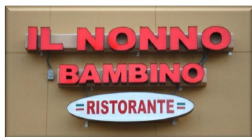
Figure 18-10: Raceway-mounted Channel Letter Sign
