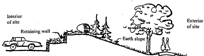
EARTH BERM WITH RETAINING WALL
