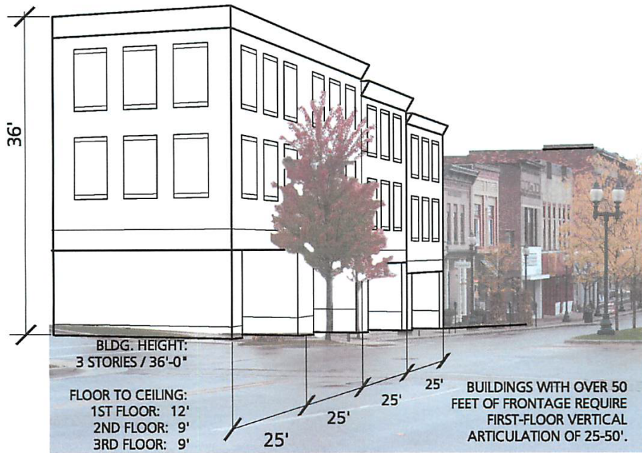
EXISTING CITY BLOCK WITH POSSIBLE THREE-STORY BUILDING
