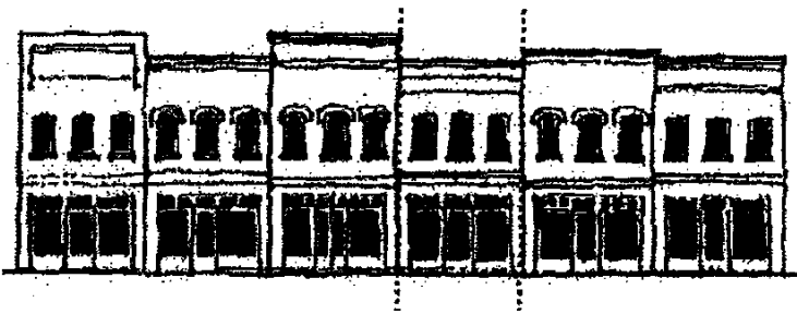
Individual storefronts, arranged in regular bays, 20 to 30 feet intervals.
