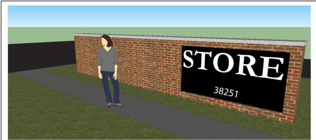
Monument Signs - the total sign area shall be no more than four times the sign surface display area. In this example, a 32 square foot sign surface display (area in black with white letters) is shown on a 128 square foot sign (5' x 25.6').
