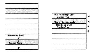
27.02:13. Lot space requirements for the layout of the parking at various angles shall be in accordance with the following minimum regulations (see ADA regulations, § 27.02:12):
