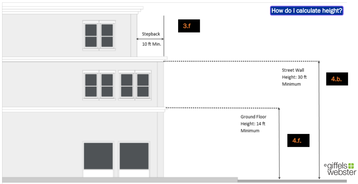
Figure 98-3.14D.3. Stepbacks, Street Walls, and Ground Floor Minimums
