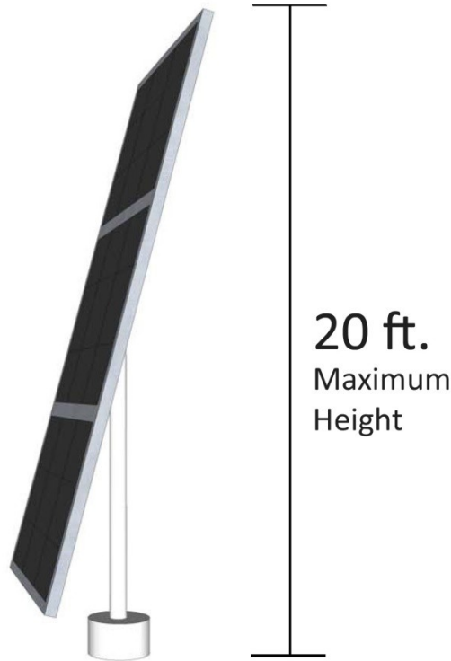
Ground-Mounted Collector Example
