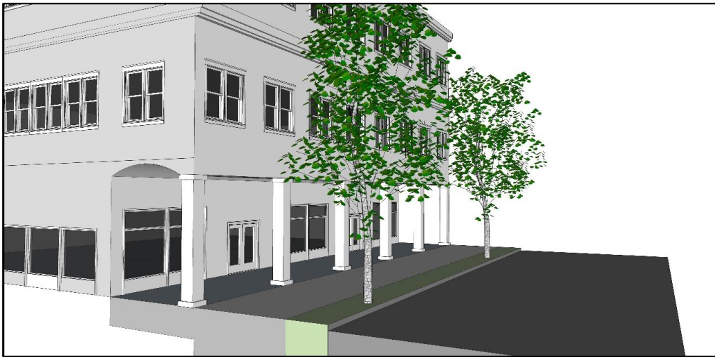
Figure 60-123 (j)(2)(b) below: Arcade section view shows the recessed pedestrian walkway and the upper floor area above. The entire structure is on private property, and the columns and upper floors extend to the front lot (build to) line.
