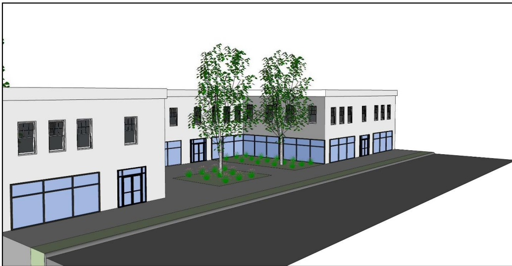
Figure 60-123(j)(3)(b) below: Forecourt section view shows the relationship of the development lot to the right-of-way. The courtyard area is not visible from this angle, as it is behind the portion of the building placed at the build-to line.
