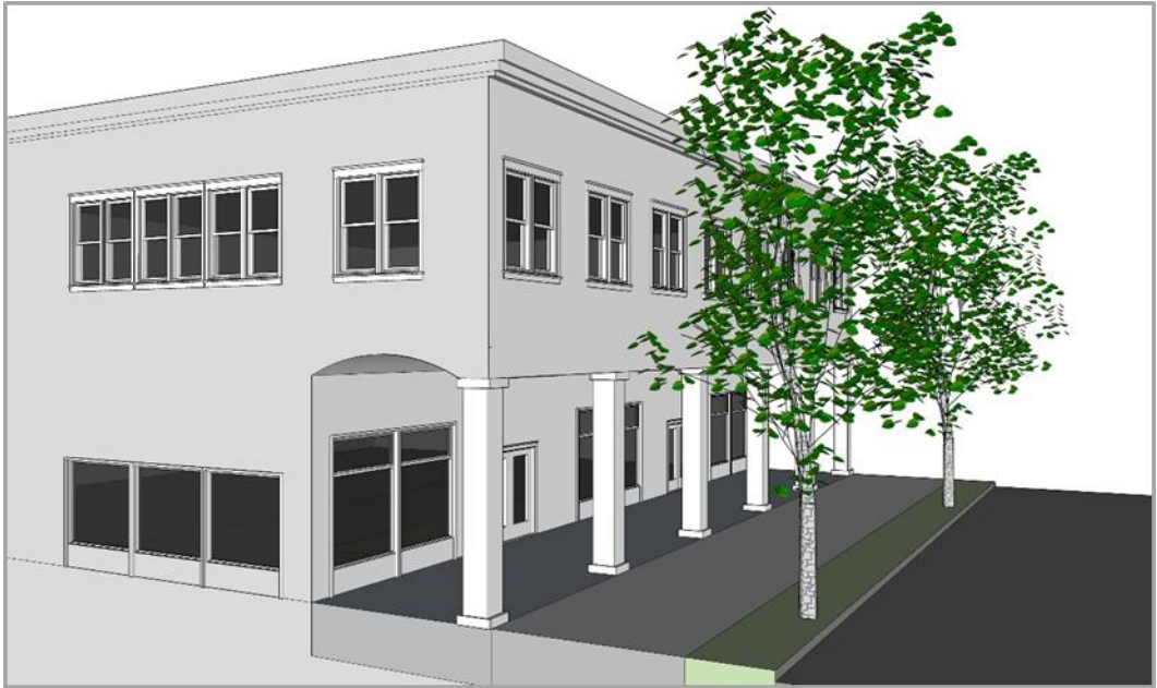
Above: Arcade axonometric view shows how the building design creates a recessed ground floor shopfront area. The upper floors project over the pedestrian walkway to the front lot (build-to) line.
