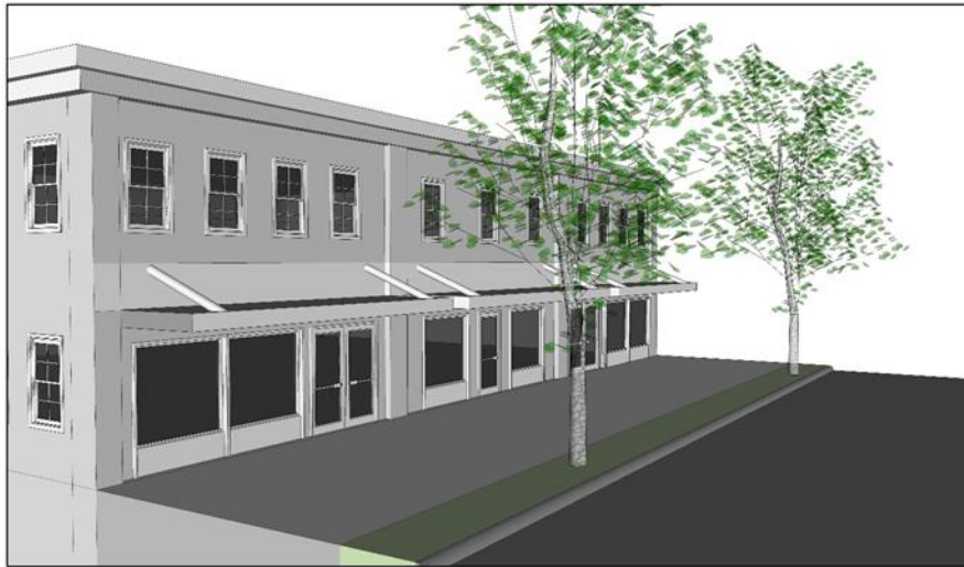
Above: Shopfront axonometric view illustrating pedestrian-oriented storefront that encourages walking throughout the BD District. The storefront glazing, which allows views inside the building, is a critical element that encourages pedestrians to stroll the District.
