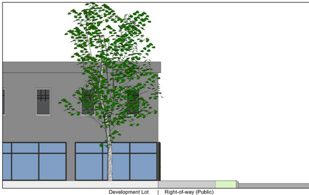
Above: Forecourt section view shows the relationship of the development lot to the right-of-way. The courtyard area is not visible from this angle, as it is behind the portion of the building placed at the build-to line.
