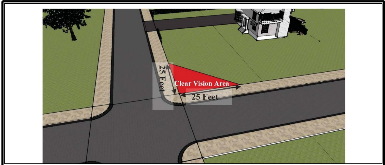
Figure VII-58 Clear Vision Area-Street Intersection
