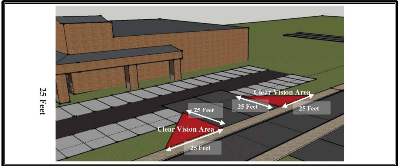
Figure VII-60 Clear Vision Area-Vehicular Access Drives
