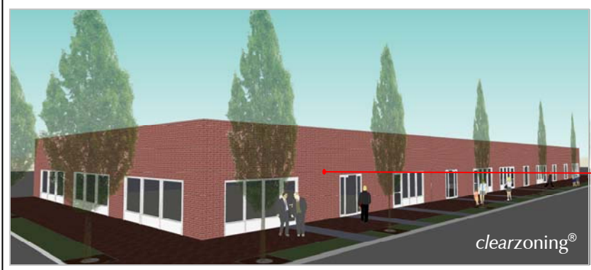
FIGURE 3.1.22.G.ii BUILDING FACADES Buildings must provide visual interest through a change in façade articulation, breaks, columns, height changes, or changes in color, texture, or pattern.
