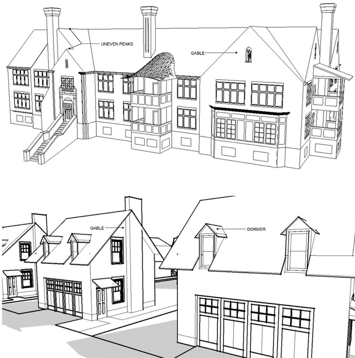
Figure 8-7: Examples of Architectural Features
