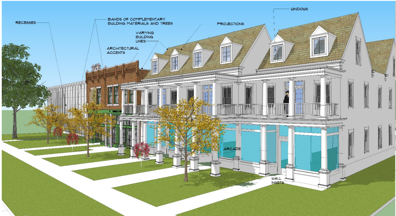
Figure 8-6: Examples of Architectural Features
