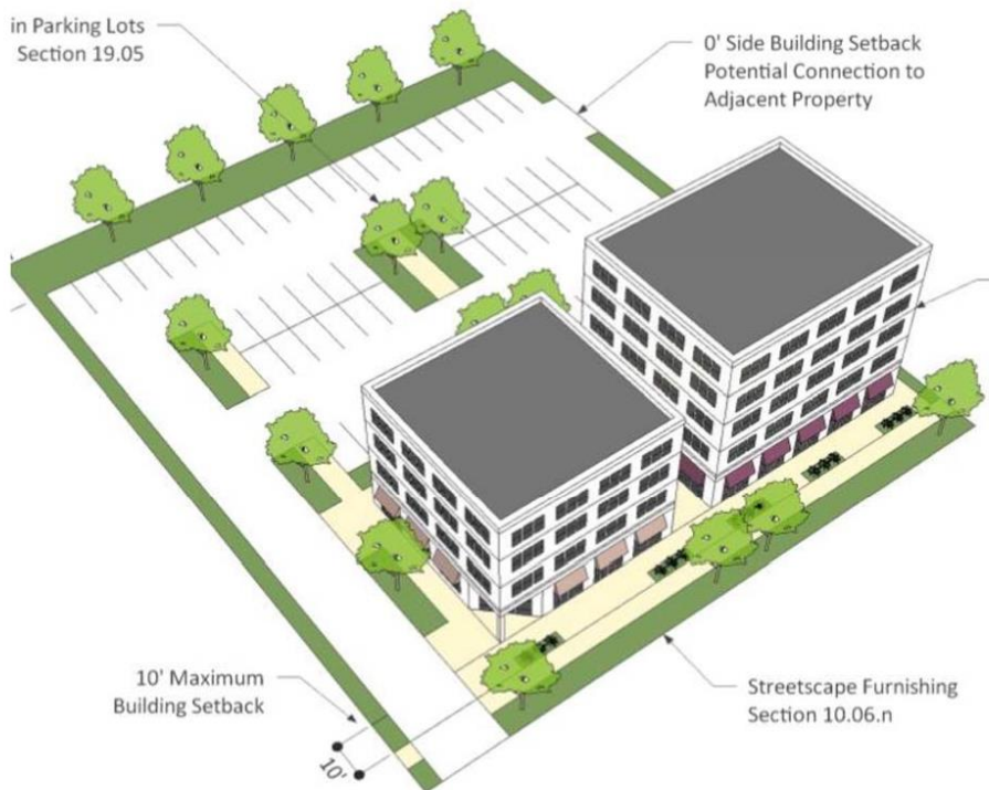
Figure 4. Shared Parking Area and Driveway
