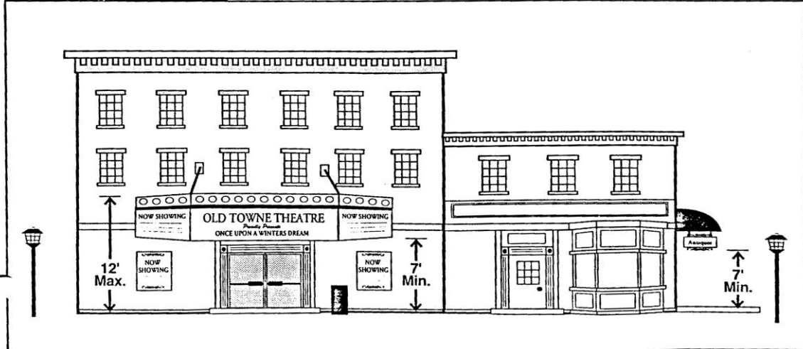
Figure (4)(m) Marquee Sign
