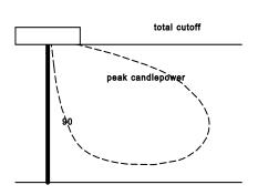
Cutoff Type Luminaire: a luminaire with elements such as shields, reflectors, or refractor panels which direct and cut off the light at a cutoff angle that is less than ninety (90) degrees.
