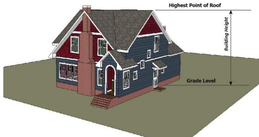
Figure 7-L: Measurement of building or structure height
