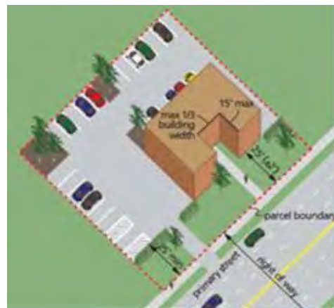
Illustration of required front building setback, maximum interior lot line setback and optional front building setback offset of 15 feet away from street.
