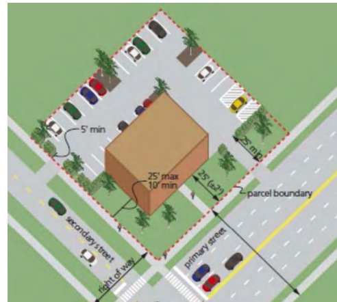
Illustration of setback requirements for a lot fronting a primary and non-primary street.
