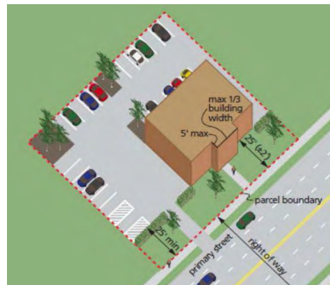
Illustration of required front building setback, maximum interior lot line setback and optional front building setback offset of 3 feet toward street.
