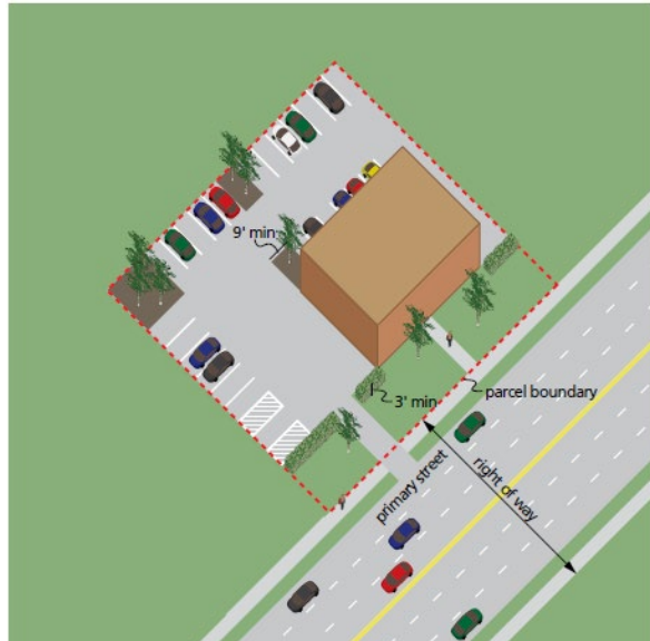
Illustration of required front yard parking lot screening and interior parking lot landscaping
