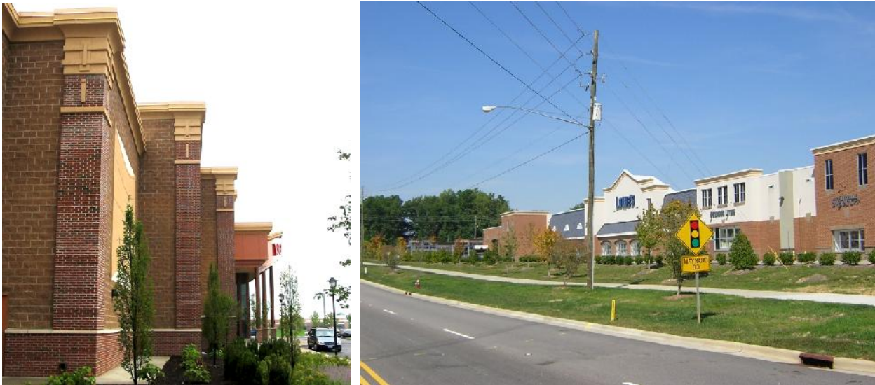
Figure 7.05-1: The buildings in the above images contain pilasters, cornices, and a series of façade setbacks (recesses) to visually break up the appearance of large facades.
