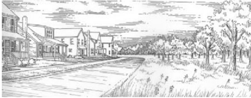
Figure 1705.B.3.a (example of a single loaded street)
