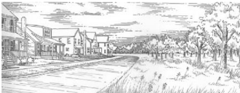
Figure 1711.B.4.a (example of a single loaded street)
