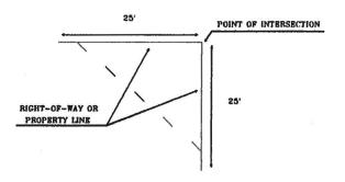
Section 304.02 CLEAR VIEW OF STREETS - Nothing greater than three (3) ft. in heights shall be located in the triangular area as shown in the above diagram.
