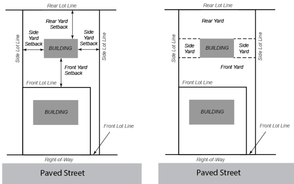
Figure 4.09-H: Typical lot lines and setback locations for a flag (panhandle) lot (left image) and typical yard locations (right image).
