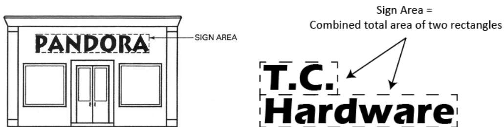
Figure 12.07-E: Illustration of sign area calculation for two differently shaped wall signs with individual letters.
