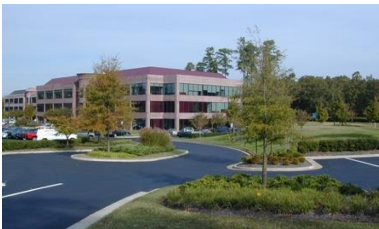
Figure 12.07-2: Landscaping and screening is intended to soften the appearance of large expanses of parking areas and can also provide areas for stormwater management.
