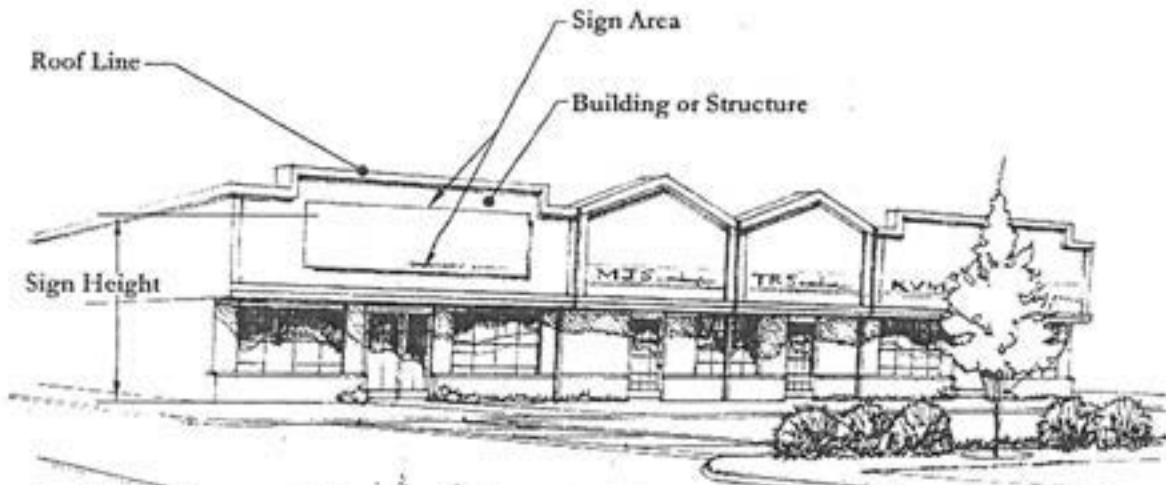
Typical building mounted sign on a multi-tenant building
