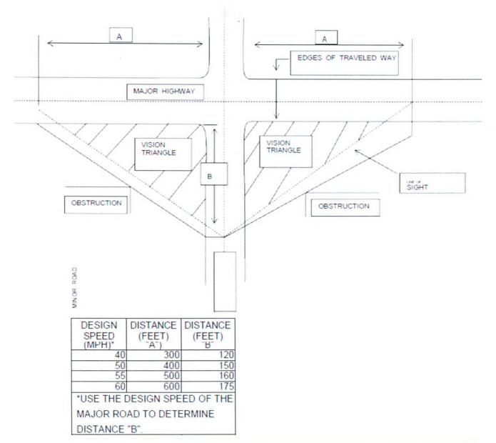
EXAMPLE: GIVEN DESIGN SPEED IS 60 MPH ON THE MAJOR HIGHWAY AND 50 MPH ON THE MINOR HIGHWAY
